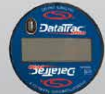
Display turns off when vibration is detected (vehicle moving) to conserve energy.
